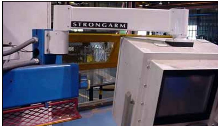
The STRONGARM touch screen swingarm has a different mounting hole configuration than the swingarm previously used. The items in SB135KIT are needed to mount the STRONGARM swingarm to your current touch screen enclosure, and onto the saw frame. To do so, you will need all of the parts supplied in the SB135KIT as shown in Table 1, the tools listed in Table 2, and the instructions in this Service Bulletin.
